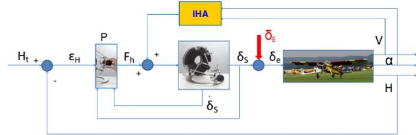
Fig. 4 - IHA Simulator Scheme. The Pilot, P, commands through the end-effector of the Omega Device the simulated aircraft.
